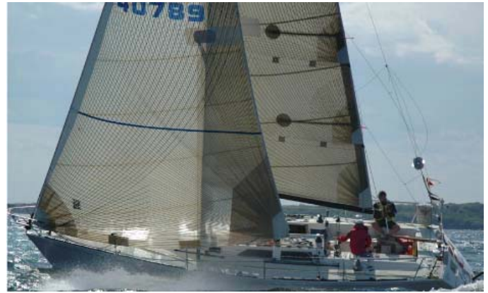
Figure 19 Carbon fiber tape reinforced laminate sails – visual metaphor of form follows force principle [UK- Halsey Tape-Drive® Sail Design]
