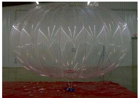
Figure 3 Lobed inflatable – ULDB test model (Raven Industries, Inc.)
